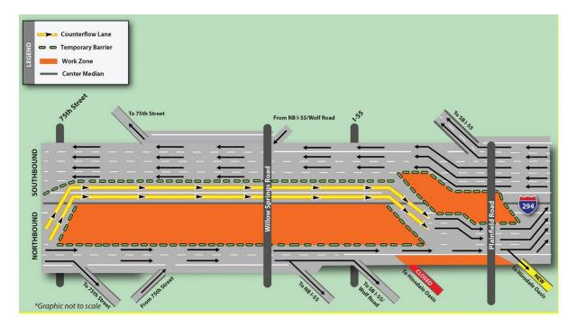
Traffic is anticipated to remain in this configuration until late February/early March. Then, as construction allows, northbound I-294 traffic between 75th Street and Willow Springs Road is scheduled to shift again with three lanes traveling on the northbound side and one lane remaining in counterflow on the southbound side.
